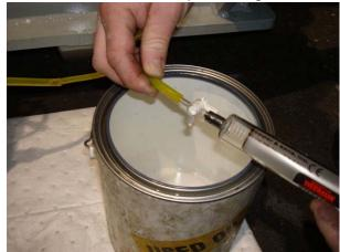
Connect hose to syringe three way valve and aim into waste bucket.
