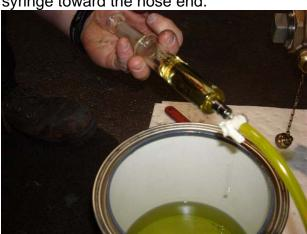
Flush the syringe three (3) times completely as shown
