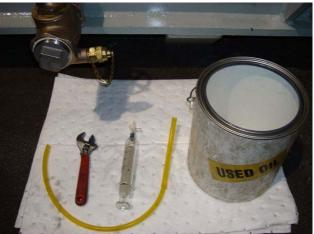
Put absorbent cloth or rag underneath work area. Layout tools and materials needed before beginning.
