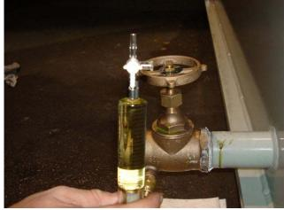
Visually inspect the oil inside the syringe sample confirming that no air bubbles exist
