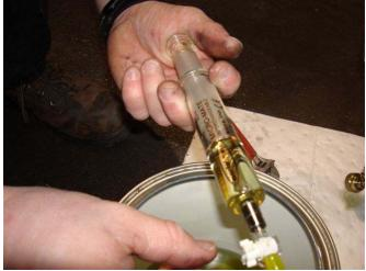
Turn the valve and flush the fluid from the syringe as shown.
