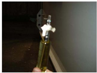
Valve shown in closed and locked position (ready to package).
