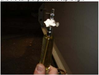
If necessary, turn valve and carefully remove any air bubbles.
