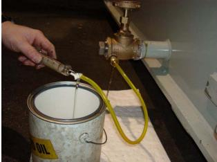
The oil is draining into waste bucket to flush contamination.
