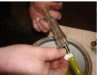
Turn valve and purge dry air from inside the syringe toward the hose end.
