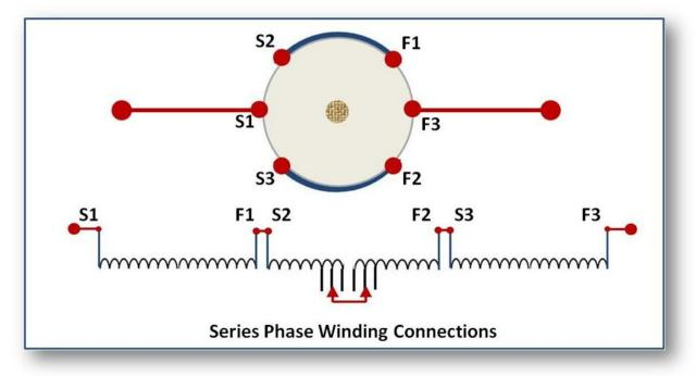
In the above illustration, the phase windings are connected in series, thereby resulting in a cumulative total of primary turns. Since the transformer low voltage
