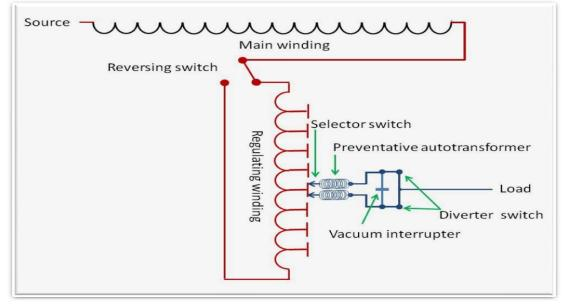
Schematic detailing key components of LTC transformer
