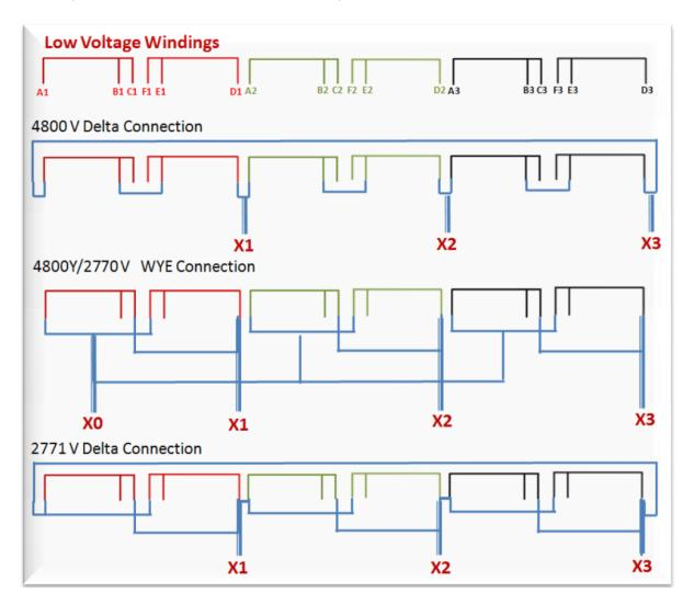
The first schematic is a copy of the LV schematic as shown on the nameplate. For clarity, each phase is displayed in a different color (A=red, B=green, C=black). Interphase connections are blue in color.
