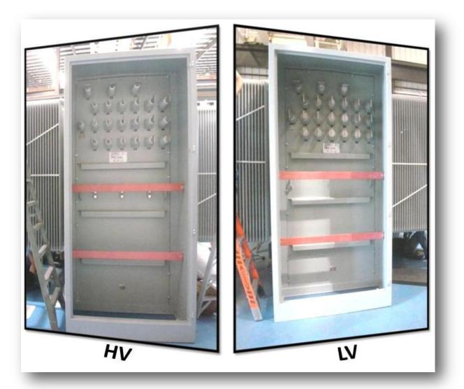
The rated amperages, winding connections, and multiple voltage requirements resulted in the decision to terminate all winding starts and finishes externally via bushings where they could be connected to provide a wide variety of inputs and outputs.
