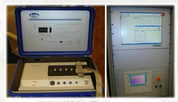
Doble partial discharge (PD) test equipment
