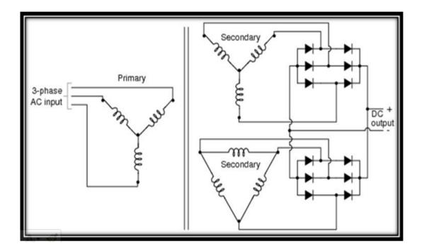
Since the ripple voltage waveforms of the two rectifiers' outputs are phaseshifted 30 degrees from one another, their superposition results in less ripple than either rectifier output considered separately since the output has now been increased from 6 pulse to 12 pulse (see below).
