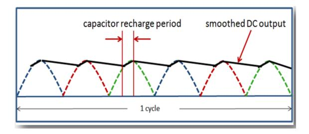
As the diagram above reveals, an increase in pulses per cycle provided by a 3 phase, 6 pulse transformer output coupled with filtering capacitors dramatically reduces the ripple effect.
