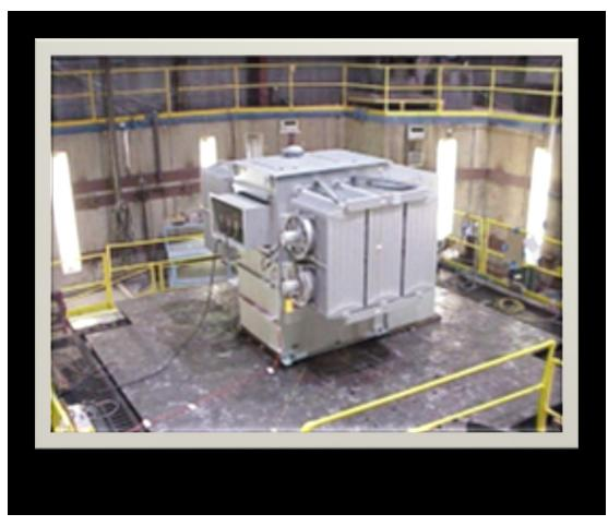
damage. The transformer passed Hi-Pot tests and IEEE Routine tests performed before and after the shake table testing, which substantiated that it withstood the shake tests without diminishing its operational performance.
