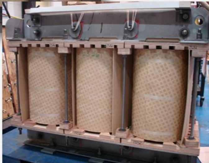
Five legged distributed gap formed cores require rectangular coil construction. This type of core and coil construction is widely used for general distribution and smaller kVA applications. The outside core legs provide a return path for magnetic flux in wye-wye connected transformers.
