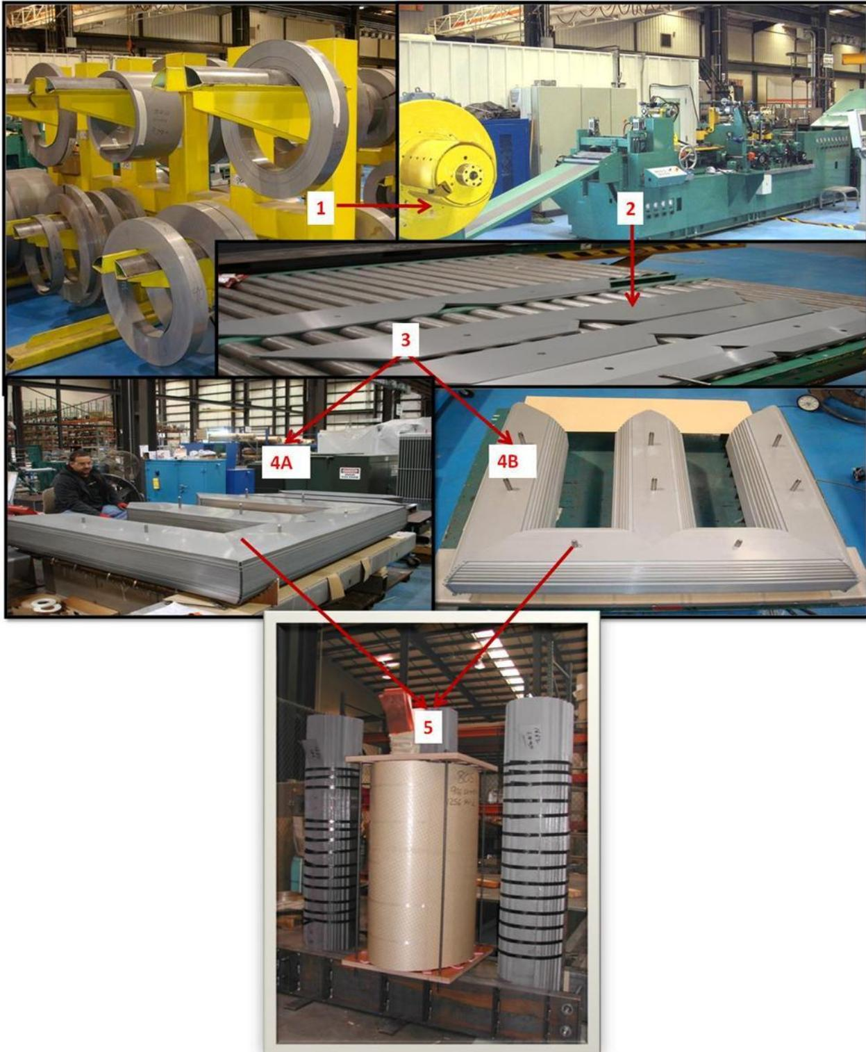
1. Varied widths of silicon steel in queue for shearing
