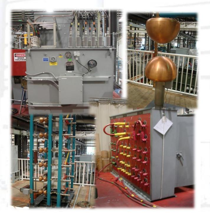
The capability to perform the required tests requires an extensive array of specialized equipment including multi-voltage test transformers, a high frequency generator, and an impulse generator.
