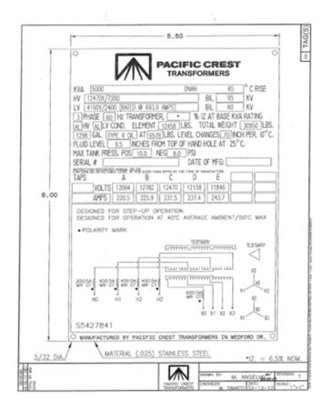
Above is an image of a nameplate drawing for a transformer recently supplied by PCT. Note the buried tertiary. The transformer was designed for generator step-up duty.
