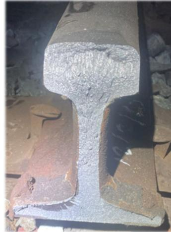
48% of broken rails are field-weld related.
