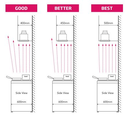
When the overhead cabinetry is constructed and installed deeper than standard, ensure the rangehood is installed as close to the front as possible. This will increase the rangehood extraction results as there is a greater coverage of the cooktop surface area.
