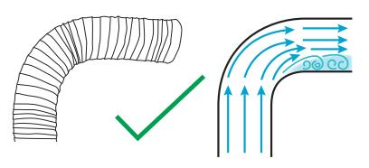
**2.** Sweeping curves and taut ducting reduces resistance and turbulence. The airflow and extraction will be more efficient and stronger.
