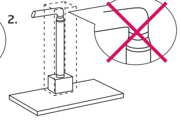
Never fit reductions next to curves or bends in the installations. They must always be in straight sections and as far as possible from the rangehood.
