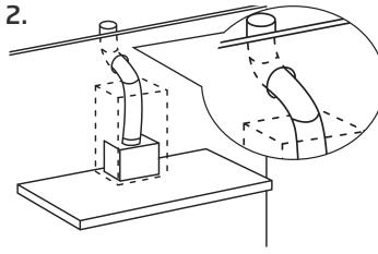
Keep the curves or bends to a minimum. If they do exist, try to keep the angles as open as possible.
