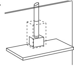
Straight ducting is the most effective installation
