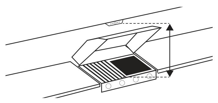
Measurements are from the top of the trivets to the lowest part of the rangehood, including the button controls.
