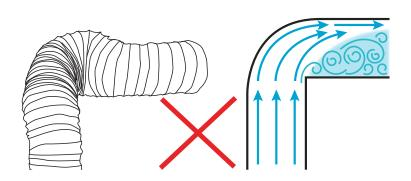
**1.** Crushed or kinked ducting creates sharp corners that creates turbulence. This reduces the size and efficiency of the ducting, lowers extraction and may cause excessive noise.
