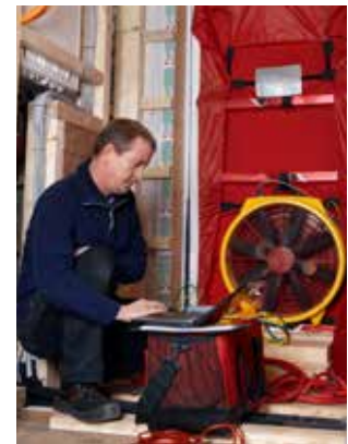
Blower-Door opening pressure >65 Pa prevents leaks, ensuring environmental control.
