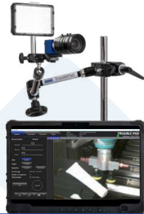
TroublePad high-speed camera with lighting on its mounting arm
