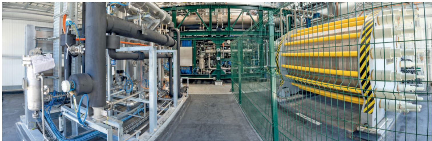
Interior of the 2.5 MW electrolyzer installed by Petronor.
