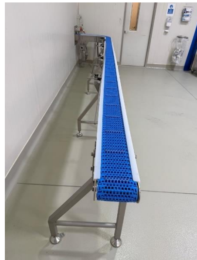
16794s – Conveyor - Belt
