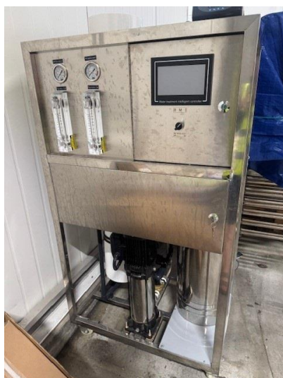
16917s – Reverse Osmosis Plant
