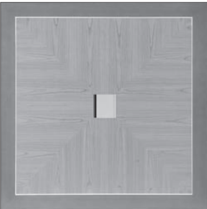
Option C Flat cut, Book-matched veneer (veneer pattern as shown), stained edge, natural finish centre, 1/4" polished aluminum reveal.
