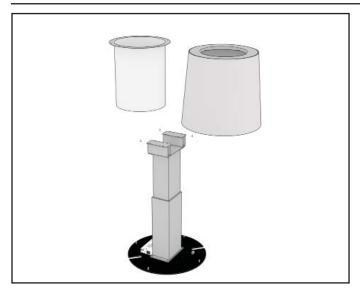
**Step 1**Remove the metal shroud and leather base from the column.
