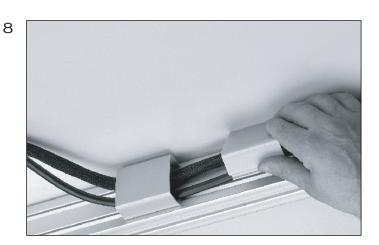
• Using wire management "U" clips, store and route cables to bases along the rails.
