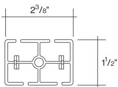
The Vox® Linked Cable Conduit is comprised of a series of plastic elements that are divided into 4 cavities.
