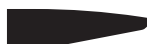
Camber Edge "CE" 8" radius required for soft corner tops 5% upcharge laminates not available
