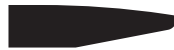
Camber Edge "CE" 8" radius required for soft corner 5% upcharge laminates not available
