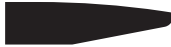
Camber Edge "CE" 8" radius required for soft corner 5% upcharge laminates not available
