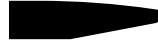
Camber Edge (CE) 8" radius required for soft corner tops 5% upcharge laminate not available
