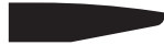
Camber Edge "CE" 8" radius required for soft corner tops 5% upcharge laminate not available
