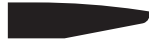
Camber Edge "CE" 8" radius required for soft corner tops 5% upcharge laminate not available
