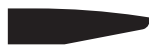
Camber Edge "CE" 8" radius required for soft corner tops 5% upcharge laminate not available
