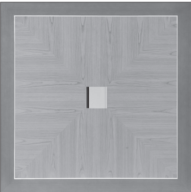
Option C Flat cut, Book-matched veneer (veneer pattern as shown), stained edge, natural finish center, 1/4" polished aluminum reveal.
