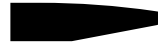
Camber Edge (CE) 8" radius required for soft corner tops 5% upcharge laminates not available
