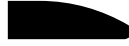
Flowform Edge (FF) 5% upcharge laminates not available not compatible with soft radius corner tops
