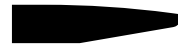
Camber Edge (CE) 5% upcharge laminates not available Camber Edge requires an 8" radius for "Soft" corners
