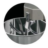
Breaker bar as standard; helps form and improve the **structure** of the dough during mixing.
