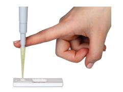
While strip test develops, enter the sample ID into Vertu TOUCH reader.
