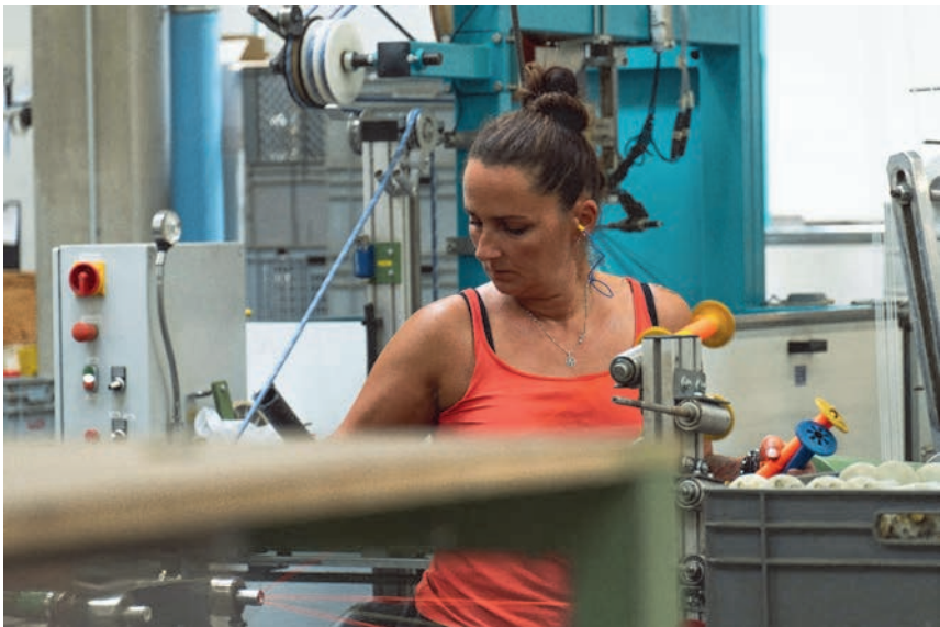
In a rope factory, safety is provided by cages around the moving parts of machines. However, it is a noisy environment, so ear protection is necessary. Teufelberger, Czechia 2023.
