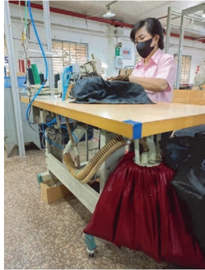
Overlock machine with vacuum to remove dust and lint. QVE, Vietnam 2023
