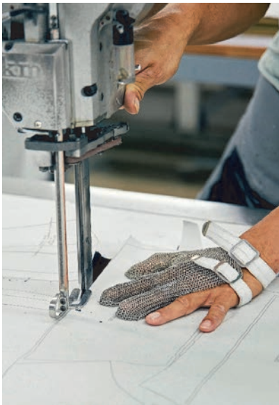
Chain mail glove to protect workers using reciprocating knife cutting machine. Spectre, Vietnam 2023
