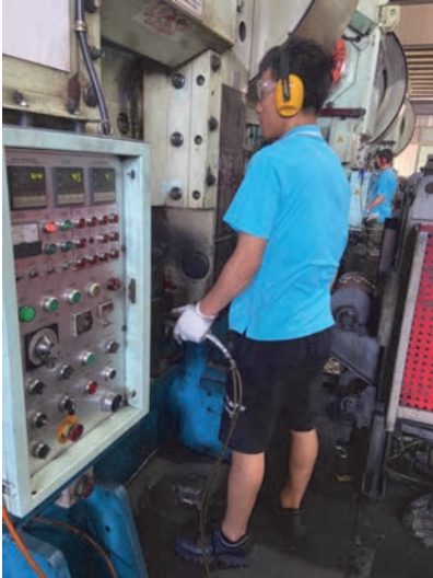
Worker using a hot forging press to make carabiners. Note the PPE – safety glasses, ear muffs, gloves and safety shoes. Also note the emergency stop switch is highlighted with a yellow ring. Carabiners Inc, Taiwan 2023
