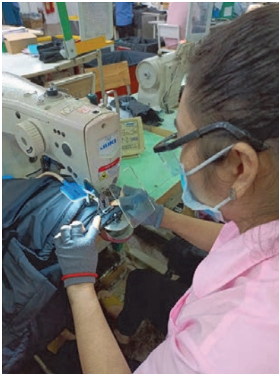
Transparent Perspex eye guard on a bar tack machine protects the operator if the needle breaks.
