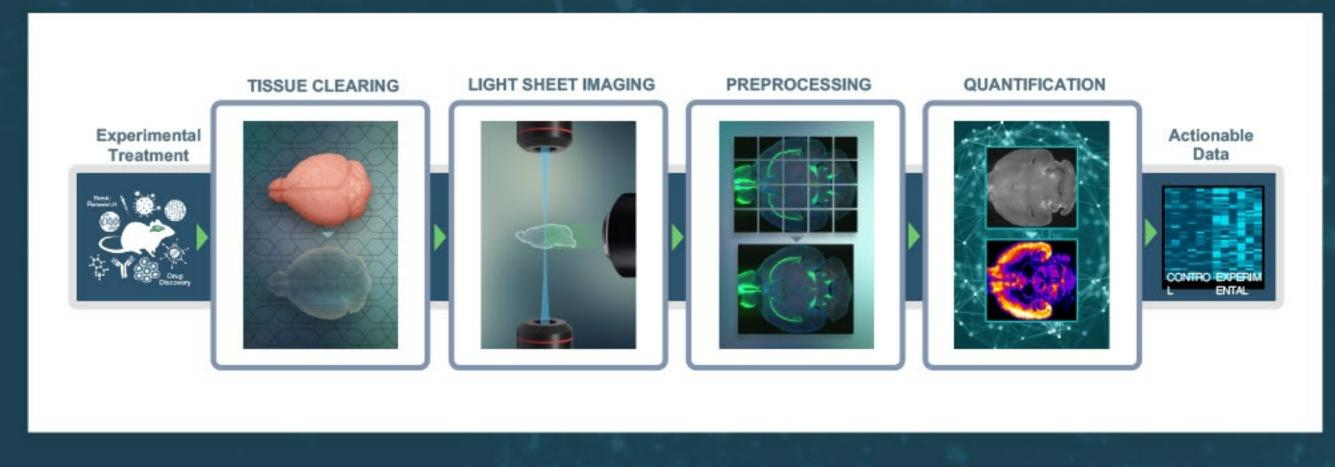
Mice are experimentally manipulated, including treatment with small molecules, antibody therapeutics, cellular therapeutics and gene therapies. Fixed and perfused brains are cleared and immunostained intact and then imaged on the ZEISS Lightsheet Z.1 microscope. After tiling and stitching in our Stitchy software, our machine learning-enabled AI-powered Voxels™ software produces actionable anatomics data.
