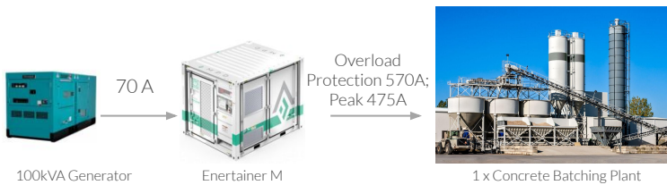
Figure 1. With 70 amps recharging from a 100kVA generator.
