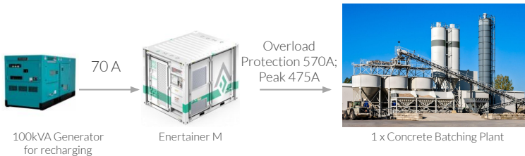
Figure 1. With 70 amps recharging from a 100kVA generator.
