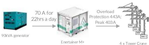
Figure 1. 'Block' diagram of the connection between the Diesel Generator, Enertainer and the loads
