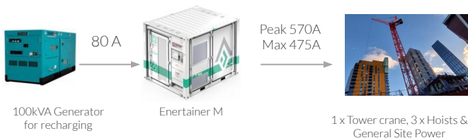
Figure 1. With 80 amps recharging from a 100kVA generator, ~7am-8pm only.
