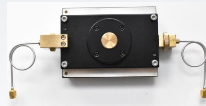
SPDR: DK/DF Test equipment Frequency : 10G、15G
