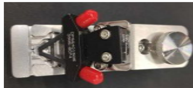
Delta L 3.0 measurement probe Frequency : 20GHZ
