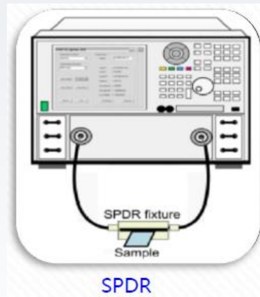
SPDR: DK/DF Test equipment Frequency : 10G、15G
