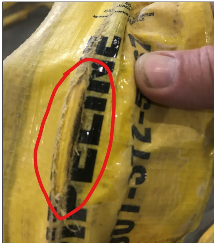
Figure 9. Abrasion Point (3) with exposed tracer wire
