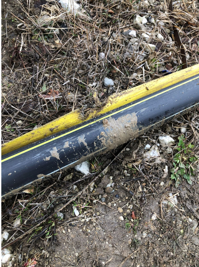
Figure 6. Field observed abrasion and material removal
