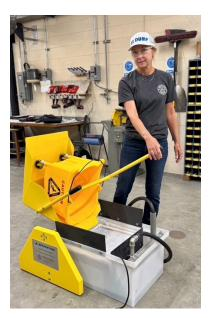
**EZ Mop Bucket Dump Station**: EZ lifting with handle and tilt mechanism, air-shock assists lift and holds bucket in place for rinsing, filter pad removes debris to prevent pipe plugging, sump pump transfers used mop water to drain or a holding tank.
