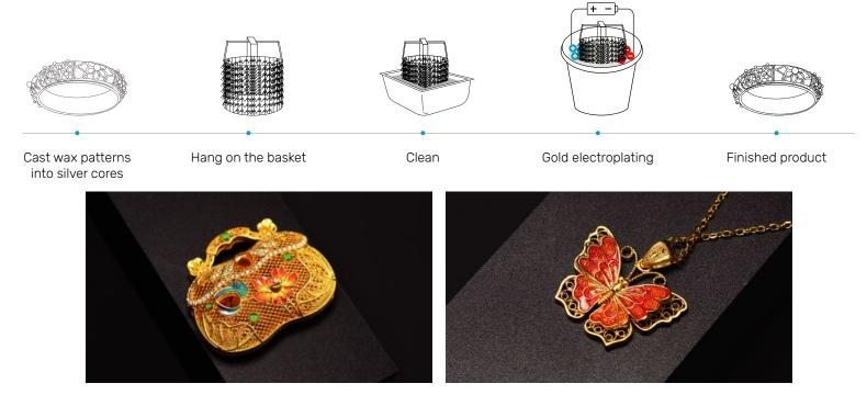
WJ530's multi-printhead system speeds up wax pattern production while ensuring consistency in silver cores, significantly boosting the efficiency of gold vermeil jewelry batch production.
