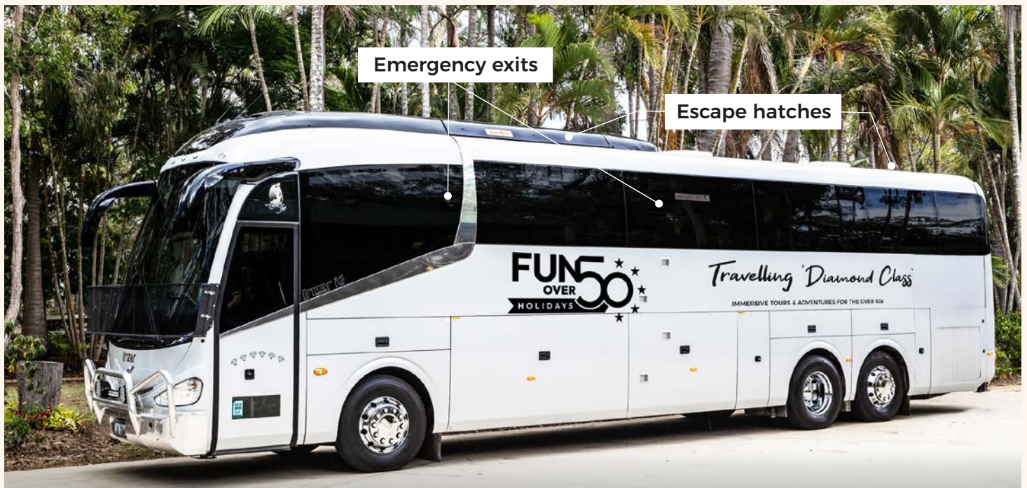
Diamond Class coach showing emergency exits and top escape hatches
