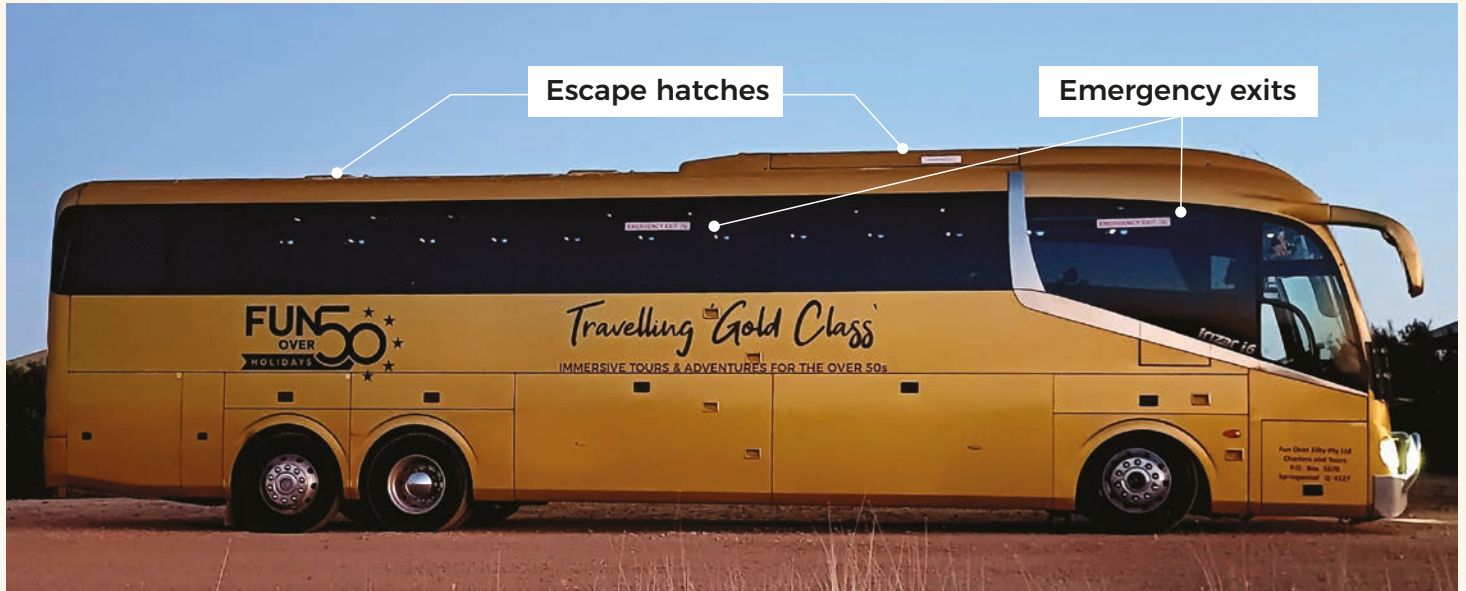
Gold Class coach showing emergency exits and top escape hatches
