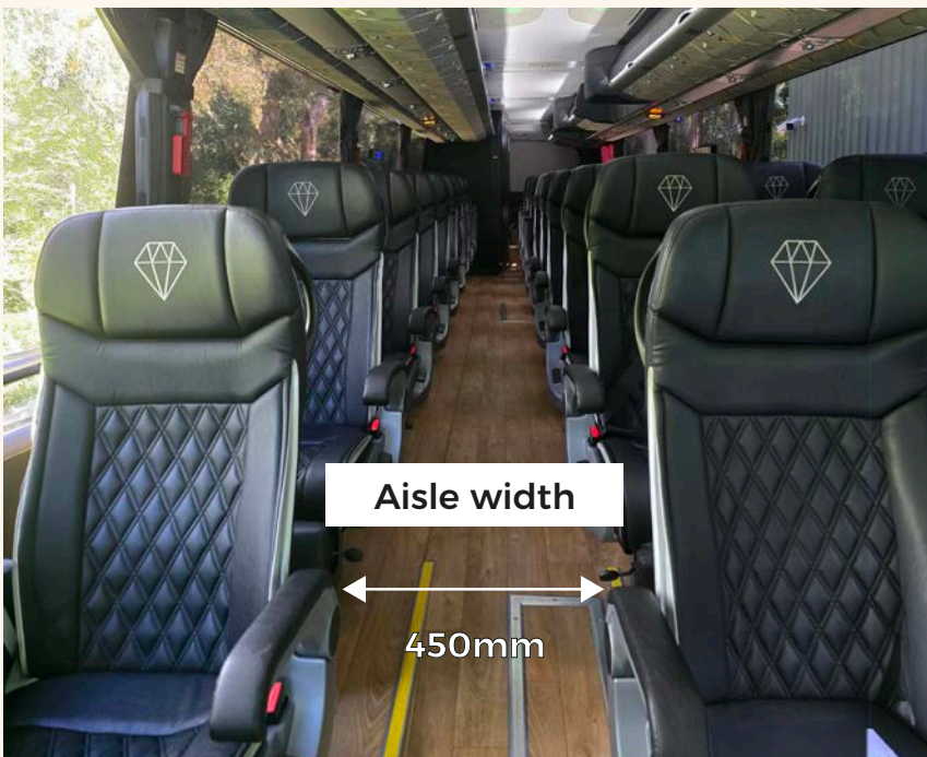
Diamond Class coach interior showing aisle width dimensions
