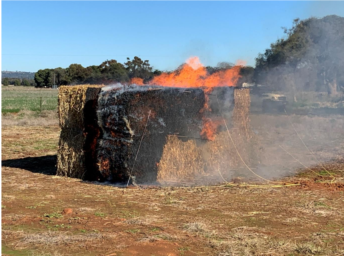
Image 2: Hay stack minutes after ignition showing location of temperature probes
