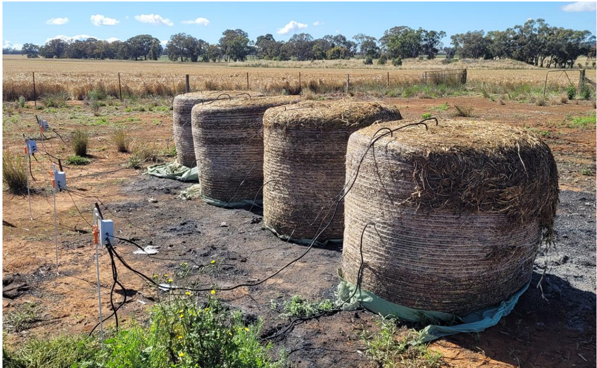
Image 3: Pea silage showing sensor installation
