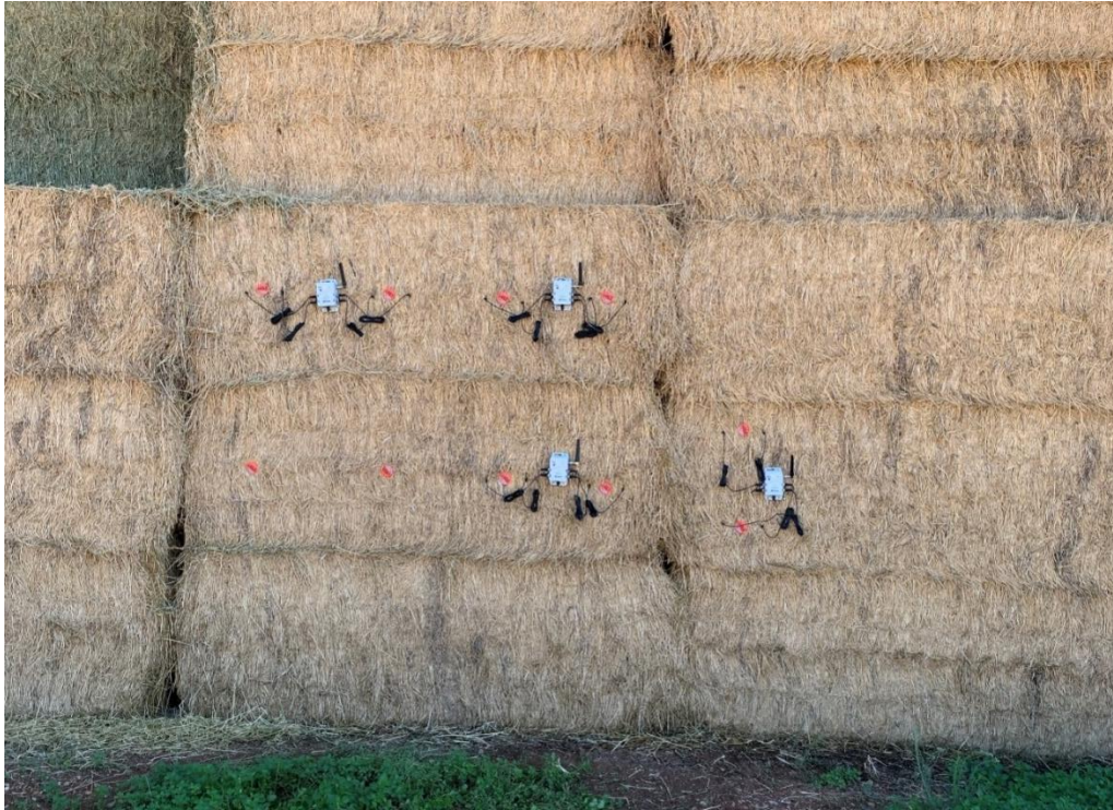
Image 1: Example of layout of the two types of temperature probes at one of the sites. Quanturi probes are orange and each of the large grey loggers has four Tinytag probes attached
