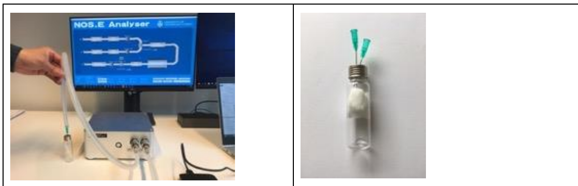
Figure 5.3.2: The head-space bottle based experimental protocol.
