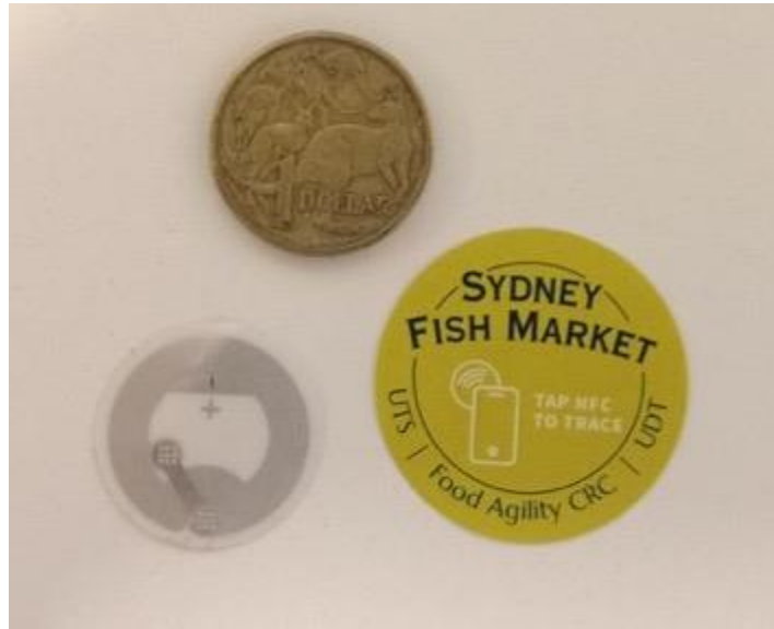
Figure 9 The smart tag with built-in NFC chip.
