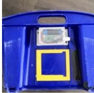
Figure 3.4.1 Installation with off-the-shelf enclosure with cable gland for the external temperature sensor
