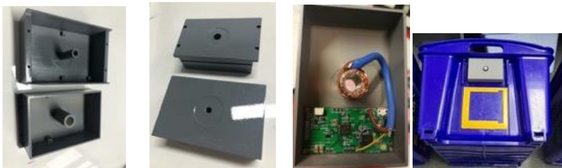
Figure 3.4.3 IoT device enclosure 3D-printed sample and installation on the fish box
