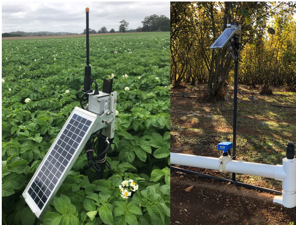
Figure 7 WildEye logger a) data logger, solar panel and high gain antenna b) data logger, solar panel and high gain antenna plus flow meter
