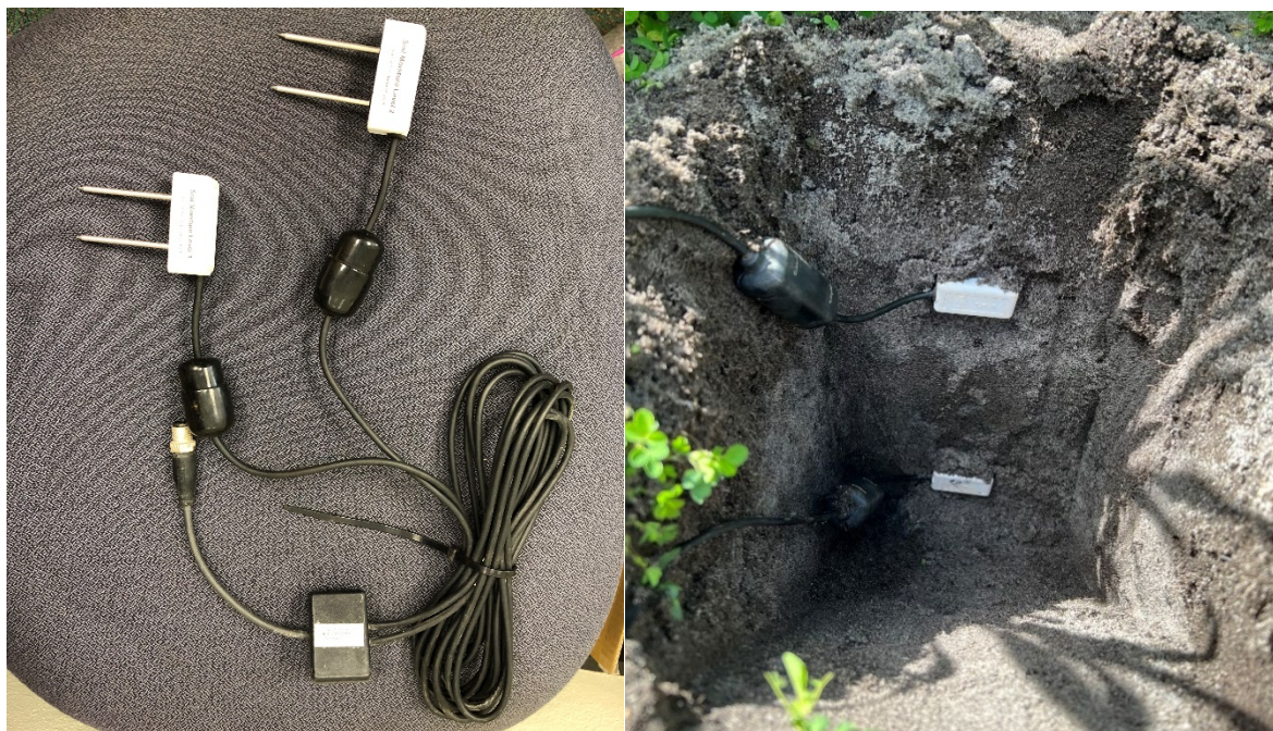
Figure 5 GS1 Teros 10 soil moisture sensor a) prior to installation b) installed
