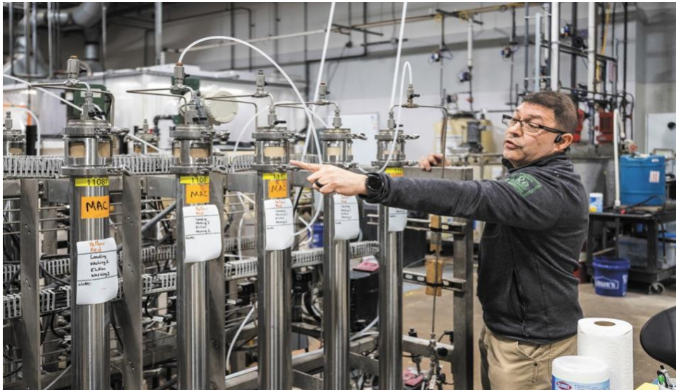
Israel Gomez, plant manager at ReElement's Noblesville facility, shows how the company processes elements like lithium, germanium, gadolinium, antimony and yttrium for reuse from recycled materials. (IBJ photo/Chad Williams)
