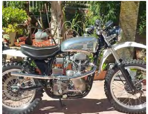
Custom Built VeloStar as seen in Motorcycle Classics, 2016 September/October Issue. 1959 Velocette MSS type S 500cc in a BSA Gold Star frame and Husqvarna telescopic front forks. $8000 | Contact: fishtailwest@gmail.com
